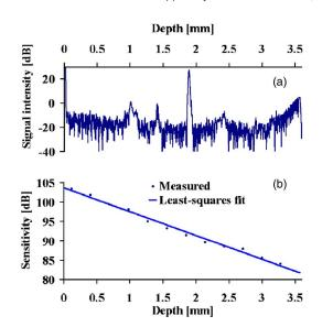
FIG. 3. (a) A typical point spread function, measured at z=1.85 mm. (b) Sensitivity degradation vs imaging depth z. The solid straight line is the least square fit of the measured data points.
