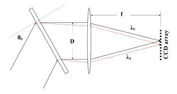
FIG. 2. Diagram of the spectrometer design.
